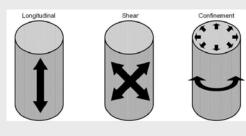
The FRP tubes reinforce the concrete, eliminating the need for steel rebar, and maximizing material efficiency.
